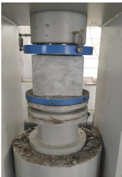
Fig.3 Compressive testing of steel fiber cube
