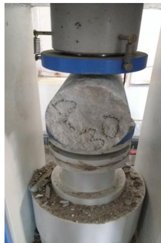
Fig.5 Split tensile strength testing of specimen
